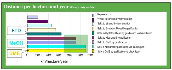
The graph shows that gasification of cellulosic biomass is the most energy efficient technology. VärmlandsMetanol AB will gasify forest residue but anticipate that Salix (willow tree) will be a common future feedstock.
